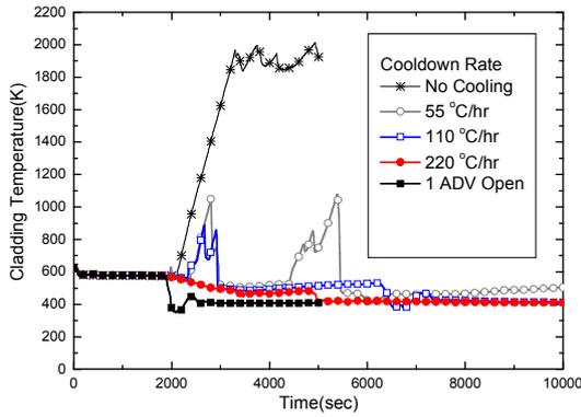
Figure 3. Peak Cladding Temperature change due to the variation of cooling rate
