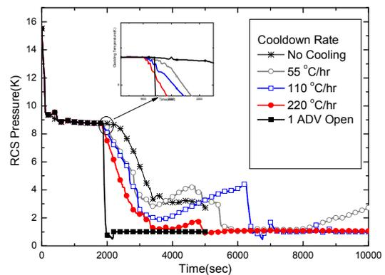
Figure 2. RCS pressure change due to the variation of cooling rate
