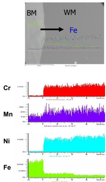
Figure 4. Element distribution line scan across the weldment .
