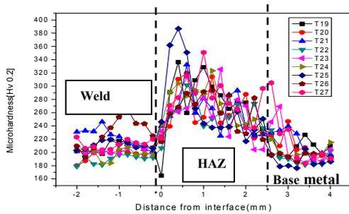
Figure 2. Micro vickers hardness distribution to the direction of depth in temper bead overlay cross-section.
