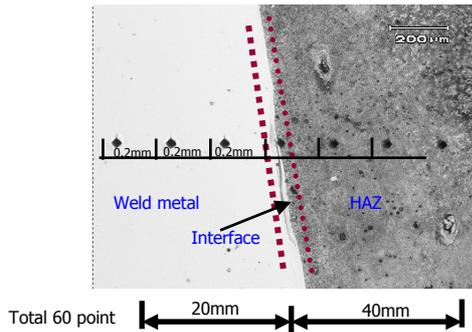
Figure 1. Photograph of indent shape formed after micro Vickers hardness test at increments of 0.2mm traversing from the weld into the base metal.
