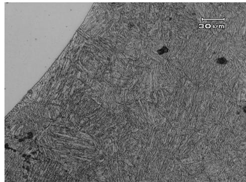
Figure 5. Optical microstructure of the HAZ in a temperbead weldment, coarse grain martensite and bainite phase.
