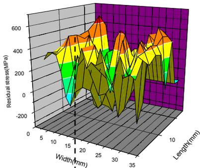
Figure 3. Residual stress distribution of T9 specimen induced by temper bead overlay welding process.
