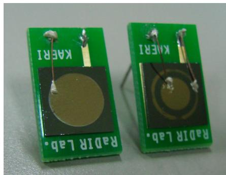
Fig. 1 Fabricated SSB radiation detectors. The right SSB has guard electrode.
