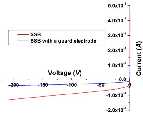
Fig. 2 The measured leakage currents of two-type SSB radiation detector.
