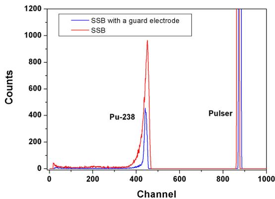
Fig. 3 The measured energy spectra for an alpha particle from  $^{238}\text{Pu}$ .
