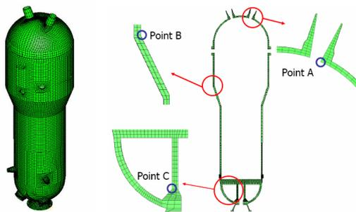
Fig. 1 The finite element model and three critical locations
