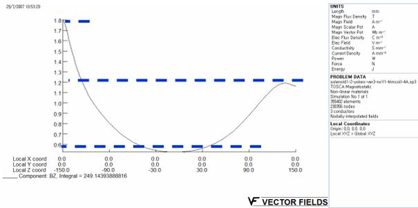
Fig. 2 Magnetid field configuration with solenoid coils for the axil field.
