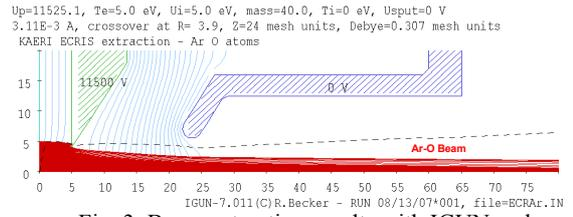
Fig. 3 Beam extraction results with IGUN code.
