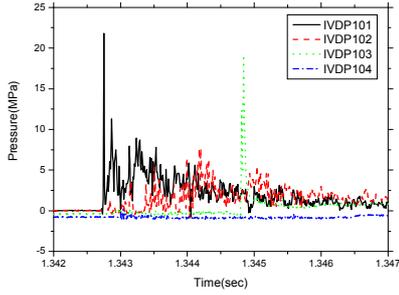
Figure 3. Dynamic pressures from the wall-mounted sensors in TROI-54.
