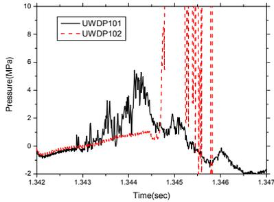
Figure 4. Dynamic pressures from the under-water sensors in TROI-54.
