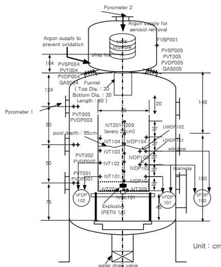
Figure 1. Schematic diagram of TROI-54.
