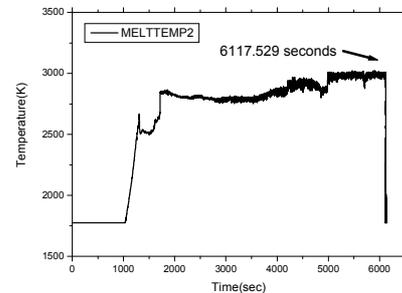
Figure 2. Melt temperature during a melting in TROI-54.
