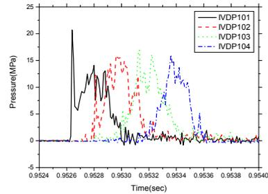
Figure 5. Dynamic pressures from the wall-mounted sensors for the calibration test.
