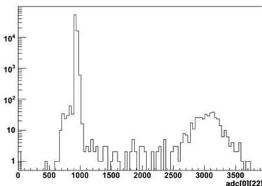
Fig. 3 Pulse height spectrum of a single strip channel measured with a proton beam.
