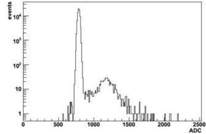
Fig. 4 Pulse height spectrum of a single strip channel measured with a  $^{90}\text{Sr}$  radioactive source.
