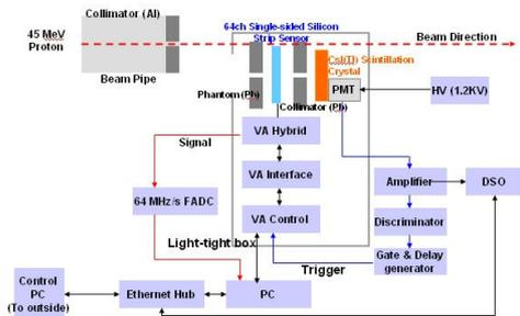
Fig. 2 Experimental setup for performance tests of the manufactured silicon strip detector with a proton beam at the KIRAMS. Sensor assembly is placed off the beam axis to protect the sensor from radiation damage.
