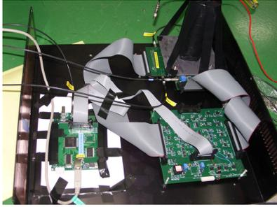
Fig. 1 Inside of the Al light-tight box which has single-sided silicon strip sensor and readout electronics assembly.
