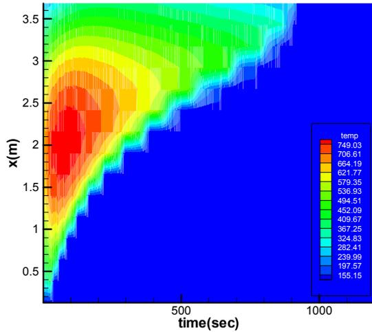
Figure 3. A heater wall temperature contour with respect to time (RBHT-C3-R1)
