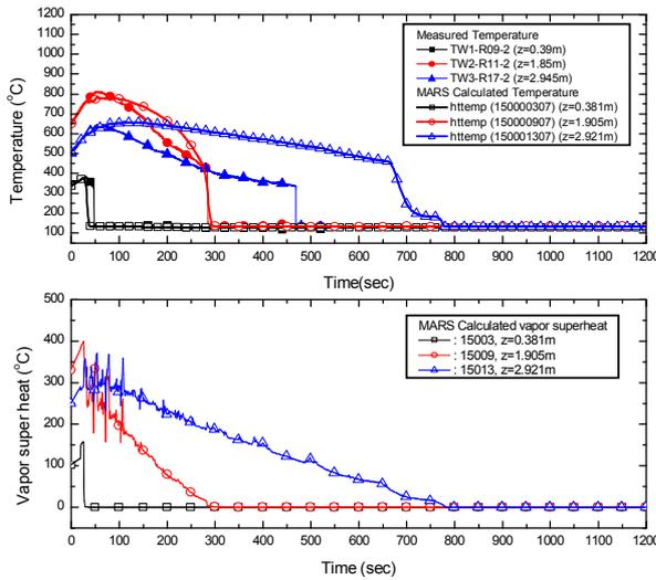
Figure 2. Trend of the heater wall temperature and vapor superheat (RBHT-C3-R1)
