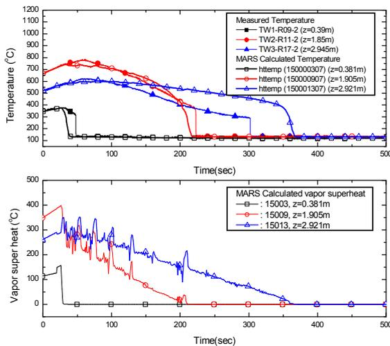
Figure 4. Trend of the heater wall temperature and vapor superheat (RBHT-C2-R1)
