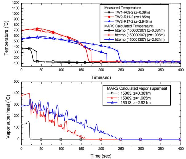
Figure 5. Trend of the heater wall temperature and vapor superheat (RBHT-C1-R1)
