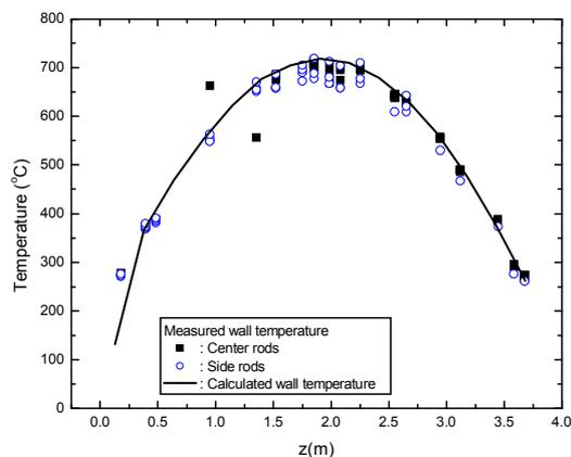
Figure 1. Initial wall temperature profile (RBHT-C3-R1)
