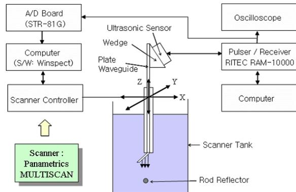
Figure 3. Experimental block diagram of transducer beam characterization
