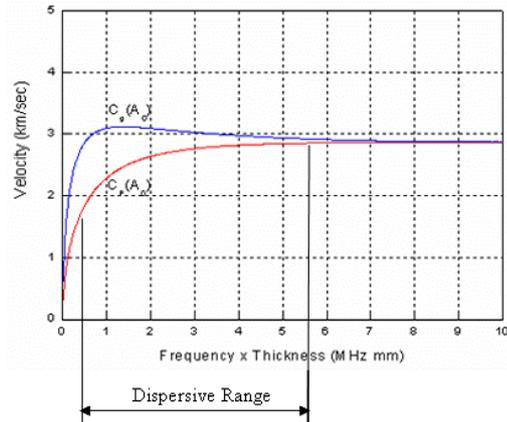
Figure 2. Dispersion curves of phase and group velocity for  $A_0$  mode
