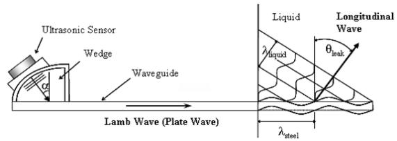
Figure 1. Waveguide sensor and leaky Lamb wave propagation
