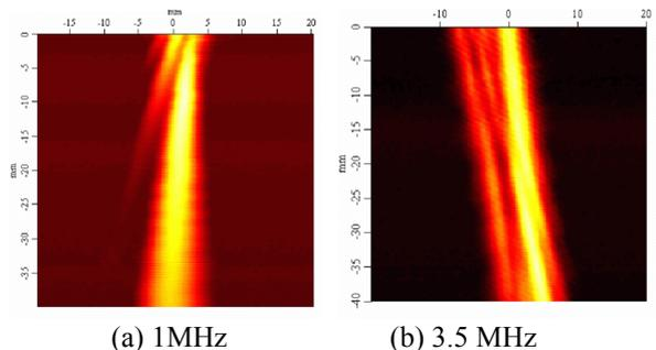
Figure 4. Transverse C-Scan beam profile images for the investigation of radiation beam steering of plate waveguide sensors
