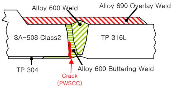
Figure 4. Schematic view of Weld Overlay Repair
