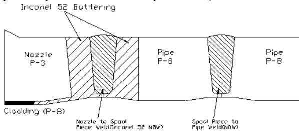
Figure 3. Schematic view of Spool Piece Replacement
