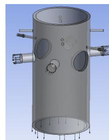
Fig. 2 Numerical model of downcomer
