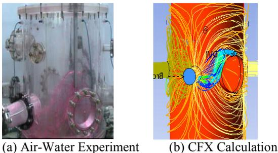
Fig.5 ECC spreading shape of the shifted DVI
