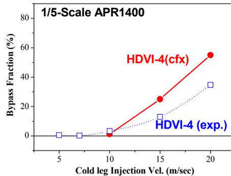
Fig.6 Direct ECC bypass fraction of the shifted DVI
