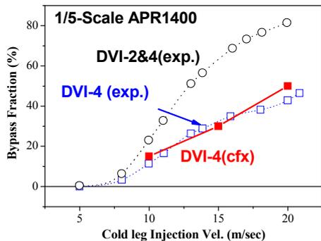
Fig. 4 Direct ECC bypass fraction
