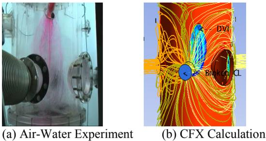
Fig. 3 ECC spreading shape of current DVI
