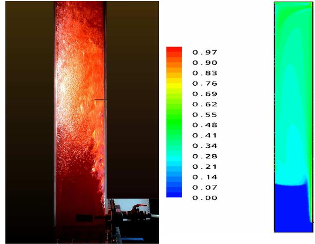
(a) Experiment (b) CFX Visualization
