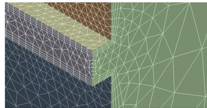
Fig. 2 CFX mesh at air INLET
