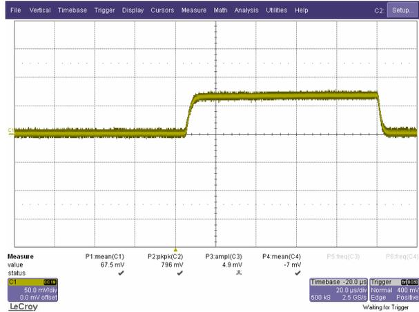
Figure 2. Cavity field profile during RF pulse test
