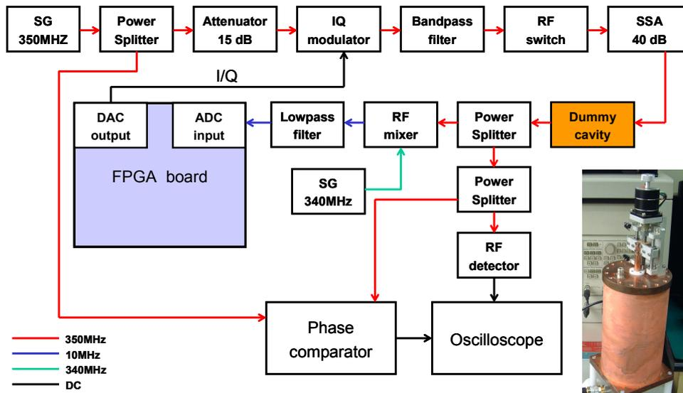
Figure 1. Schematic of the experimental setup for frequency shift measurement
