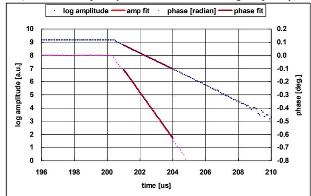
Figure 3b. Linear fitting for the decay part of cavity field (Resonant frequency is below the RF driving frequency)
