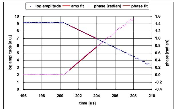
Figure 3a. Linear fitting for the decay part of cavity field (Resonant frequency is above the RF driving frequency)
