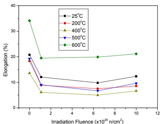
Fig. 3. Change of elongation with irradiation fluence in 10Cr-1.2Mo steel
