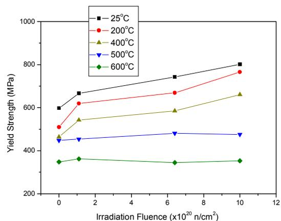
Fig. 1. Change of yield strength with irradiation fluence in 10Cr-1.2Mo steel
