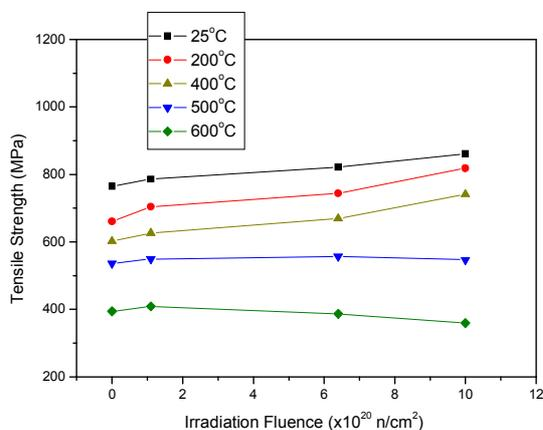
Fig. 2. Change of tensile strength with irradiation fluence in 10Cr-1.2Mo steel
