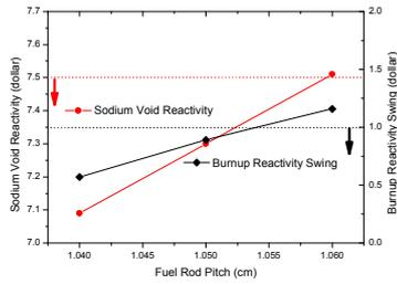
Figure 4 Effect of Fuel Rod Pitch Variation
