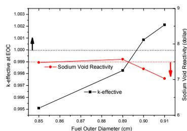
Figure 2 Effect of Fuel Outer Diameter Variation
