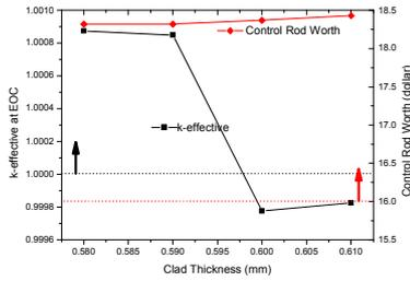
Figure 3 Effect of Cladding Thickness Variation
