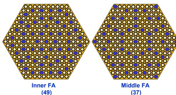
Figure 1 Non-Fuel Rods Position In an Assembly
