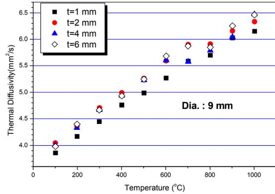
Figure 4. Thermal diffusivity of Inconel-600 with thickness
