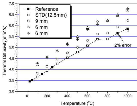
Figure 3. Thermal diffusivity of Inconel-600
