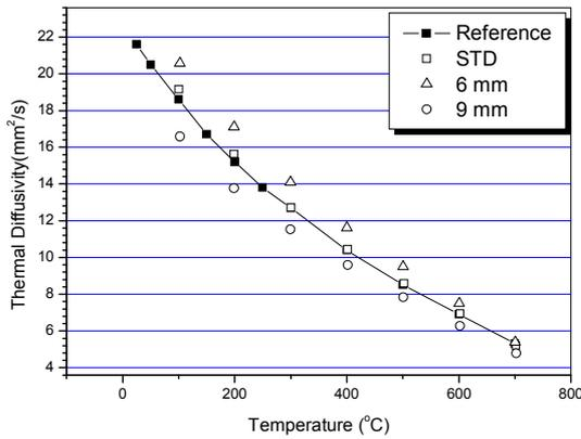
Figure 2. Thermal diffusivity of Iron
