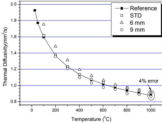
Figure 1. Thermal diffusivity of Pyroceram
