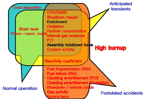
Fig.1 Categories of current safety criteria for nuclear fuel
