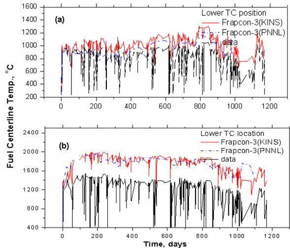
Fig.2 Changes of fuel centerline temperature in IFA-432 test rods, (a) Rod3 (small gap, 76 $\mu\text{m}$ ) and (b) Rod2 (large gap, 380  $\mu\text{m}$ ).
