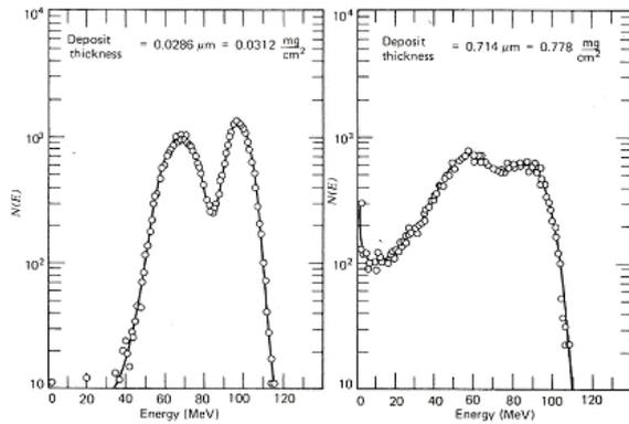
Fig. 2 Typical energy spectrum of fission chamber
