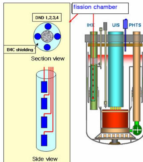
Fig. 3 Schematic location of the fission chambers
