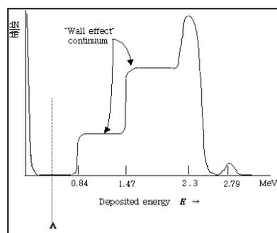
Fig. 1 Typical energy spectrum of BF-3 counter
