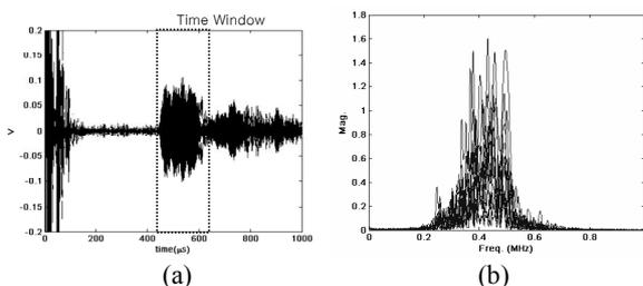
Figure 4. (a) inter-element fired signals scattered from the through-wall hole and (b) its frequency spectrum
