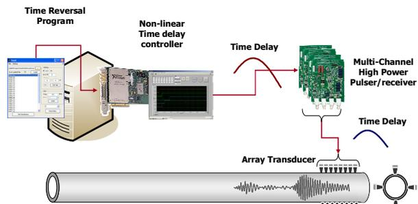
Figure 1. Schematic diagram of the ultrasonic guided wave system
