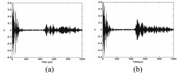
Figure 5. Guided waves reflected from the through-wall hole: (a) without time delay and (b) with time delay calculated by the D.O.R.T method
