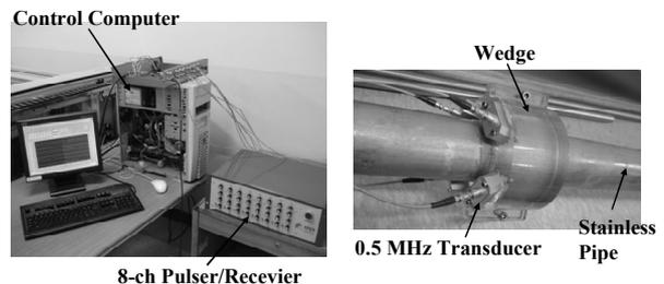
Figure 2. 8-channel pulser/receiver (left) and an array of transducers (right)
