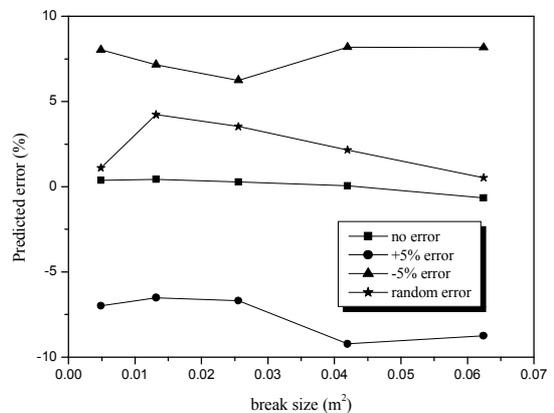
Fig. 3. Predicted errors in case measurement errors exist (hot-leg LOCA).
