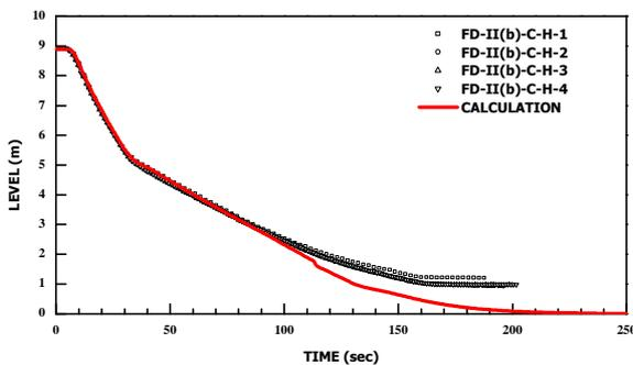
Fig. 3. Prediction of tank water level
