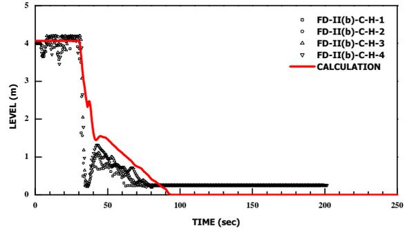
Fig. 4. Prediction of stand pipe water level
