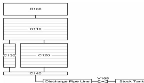
Fig. 1. RELAP5 noding for VAPER tests
