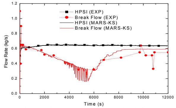
Figure 1. Comparison of HPSI and break flow
