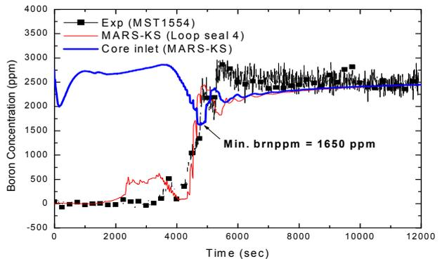
Figure 4. Boron concentration of loop seal and core inlet
