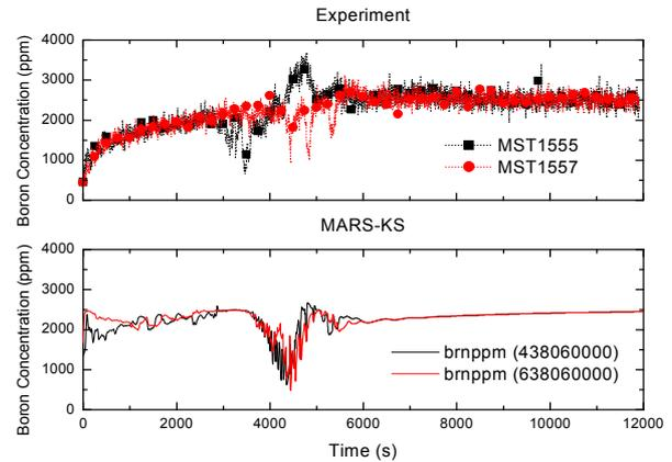
Figure 3. Boron concentration at RPV inlet in loop 2 and 4
