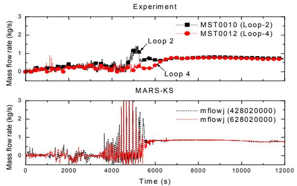
Figure 2. Mass flow rate at RPV inlet in loop 2 and 4
