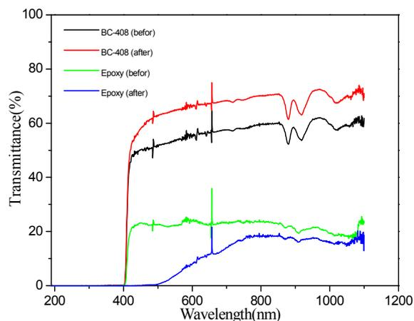
Fig. 2. Optical transmittance of the scintillation detector before and after gamma-ray irradiation.
