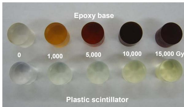
Fig. 1. The color change of the scintillation detector after high dose gamma-ray irradiation (up : epoxy base scintillator, down : plastic scintillator).
