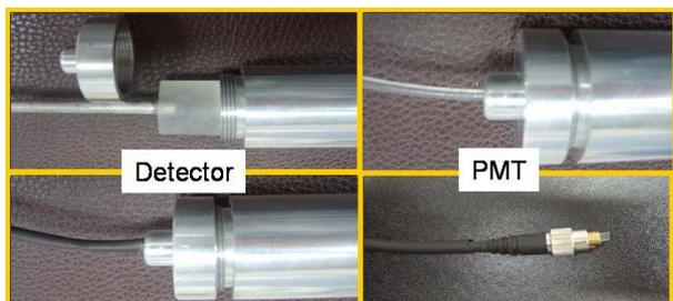
Fig. 3. The scintillation detector and PMT connected with optical fiber.
