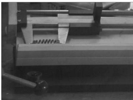
Fig. 5 Device for a spring length measurement
