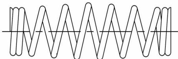
Fig. 1 Shape of the a bundle spring
