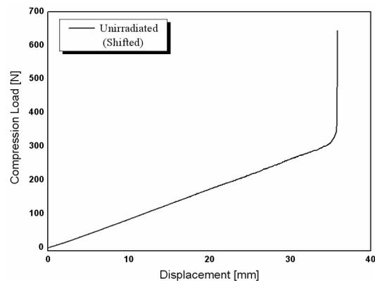
Fig. 6 Example of a test result when using the developed techniques for the unirradiated spring.
