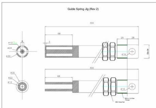
Fig. 4 Detailed dimensions of fixtures
