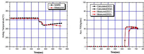
Figure 15. Ulchin 3 Hot Leg Fluid Temperature and Aux. Feed flow
