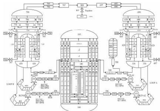
Figure 1. Ulchin 5&6 MARS-KS Nodalization
