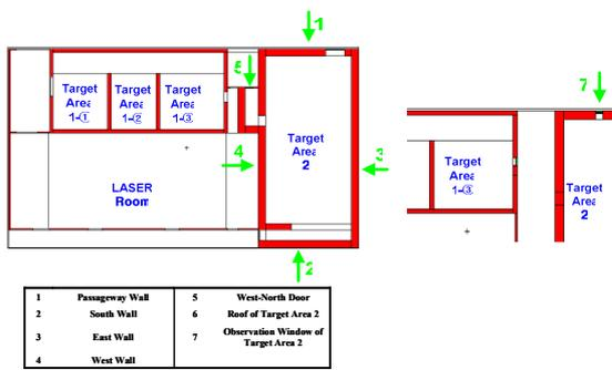
Figure 4. Dose Calculation Positions for the Experiment in Target Area 2
