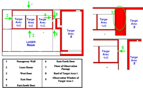
Figure 3. Dose Calculation Positions for the Experiment in Target Area 1
