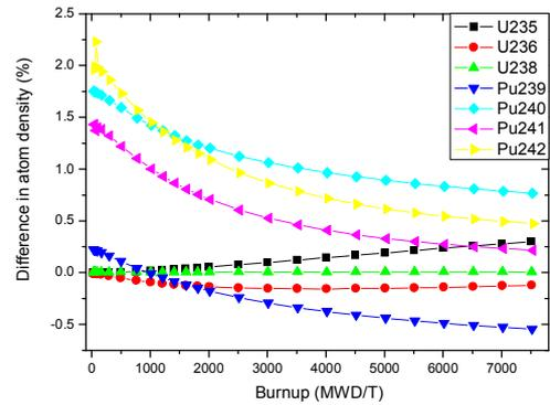
Fig. 6. Impact on the actinide density (5% creep).
