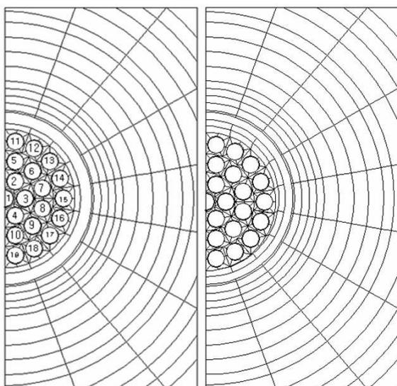
Fig. 1. Nominal and perturbed lattice models for HELIOS.
