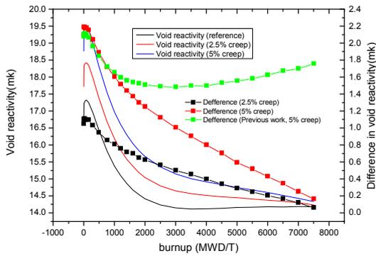
Fig. 3. Impact on the coolant void reactivity.
