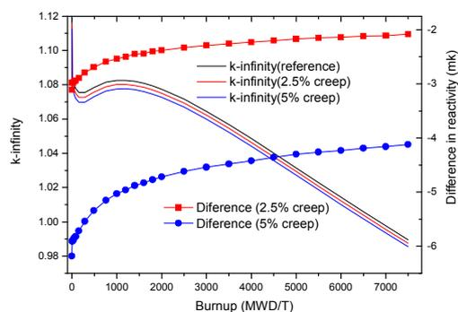
Fig. 2. Impact on the lattice reactivity.
