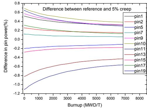
Fig. 5. Impact on the pin-power distribution.
