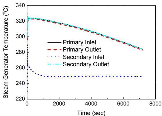
Fig. 3. Temperature variation in the primary and secondary loop of the plant
