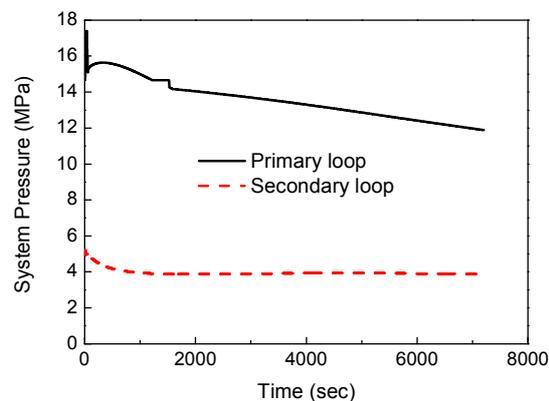
Fig. 2. Pressure variation in the primary and secondary loop of the plant
