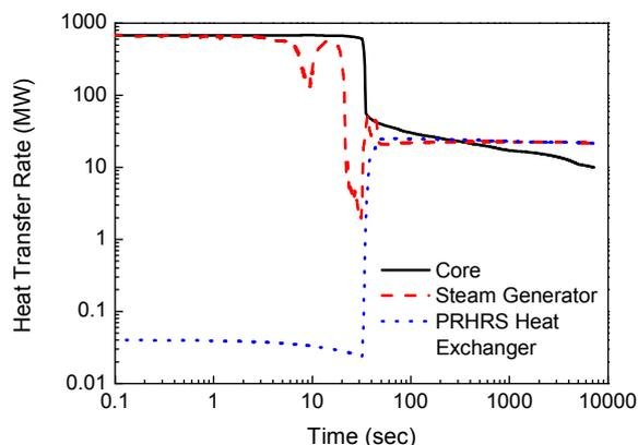
Fig. 4. Core decay power and heat transfer rate at the steam generator and PRHRS heat exchanger
