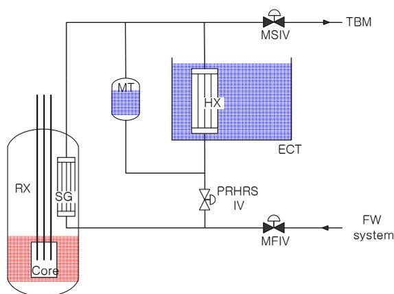
Fig. 1. Schematic diagram of the passive residual heat removal system in SMART plant (660MWt)
