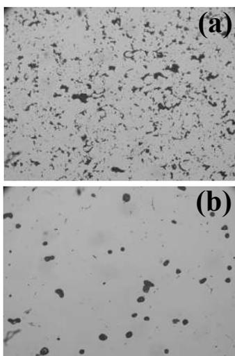
Figure 3. The pore structures of AUC  $\text{UO}_2$  pellets ( $\times 200$ ); (a) undoped, (b) 0.30 wt%  $\text{TiO}_2$
