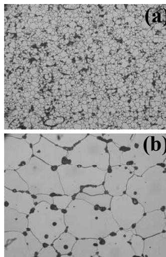
Figure 2. The grain structures of AUC  $\text{UO}_2$  pellets ( $\times 200$ ); (a) undoped, (b) 0.3 wt%  $\text{TiO}_2$
