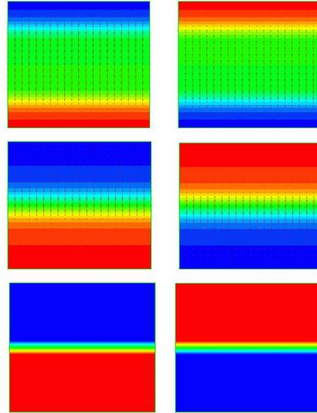
Fig. 1 Phasic distributions and velocity fields, left: liquid, right: vapor, top:  $t=2s$ , middle:  $t=4s$ , bottom:  $t=10s$
