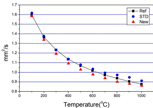
Figure 3. Thermal diffusivity of pyroceram
