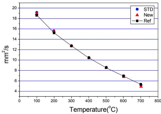
Figure 2. Thermal diffusivity of pure iron
