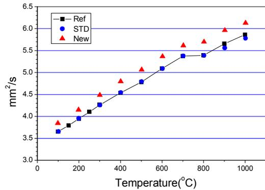
Figure 4. Thermal diffusivity of inconel-600
