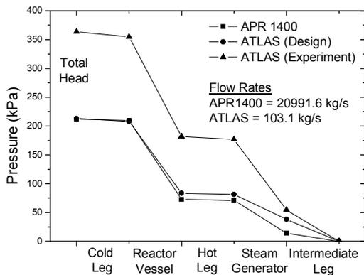
Figure 2. Pressure losses in the primary system
