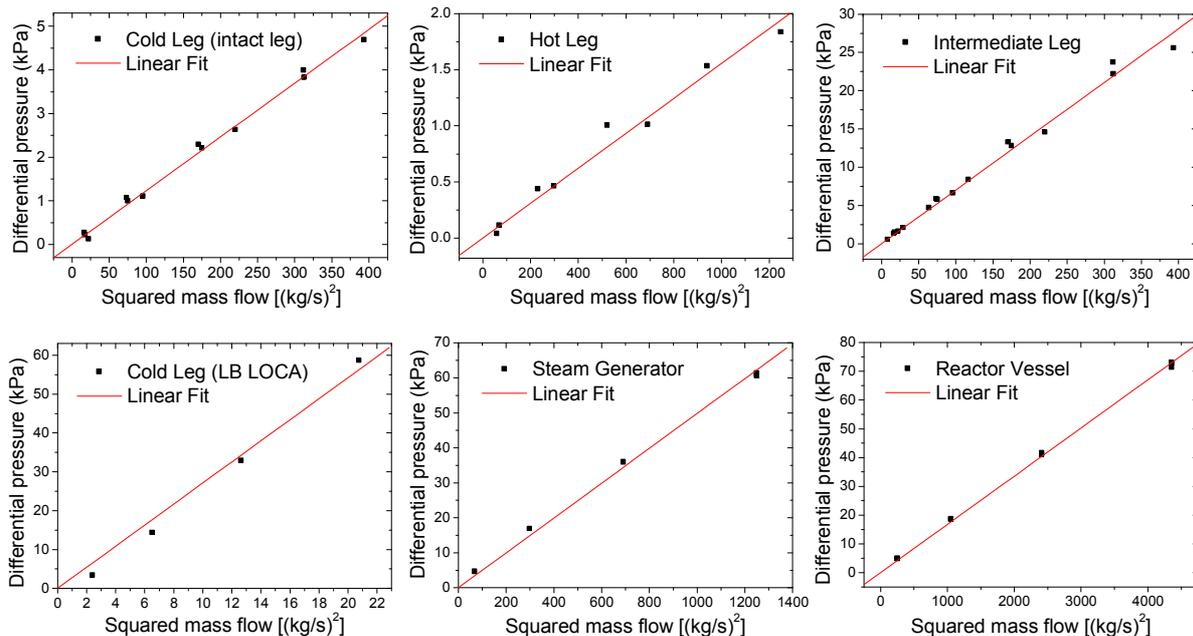
Figure 1. Pressure losses in the primary system of the ATLAS
