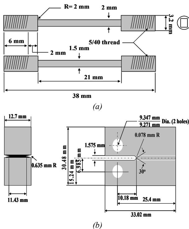
Fig. 1. Dimensions of the tested (a) tensile specimens and (b) 1/2 CT specimens.
