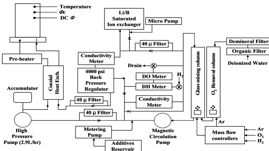
Fig. 2. Design of loop system
