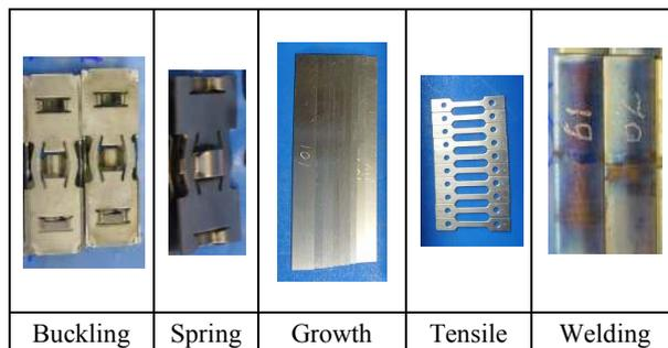
Fig. 1. KNF specimens of the parts of a fuel assembly.
