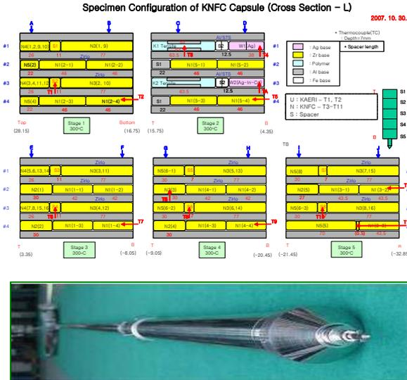
Fig. 2. Specimen configuration in the 07M-13N capsule
