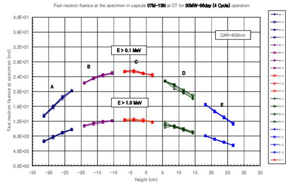
Fig. 3. The axial distribution of the fast neutron fluence of the specimens in 07M-13N capsule
