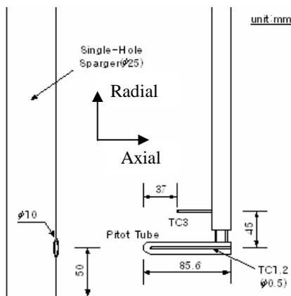
Figure 1. Single-hole sparger and pitot tube/TC
