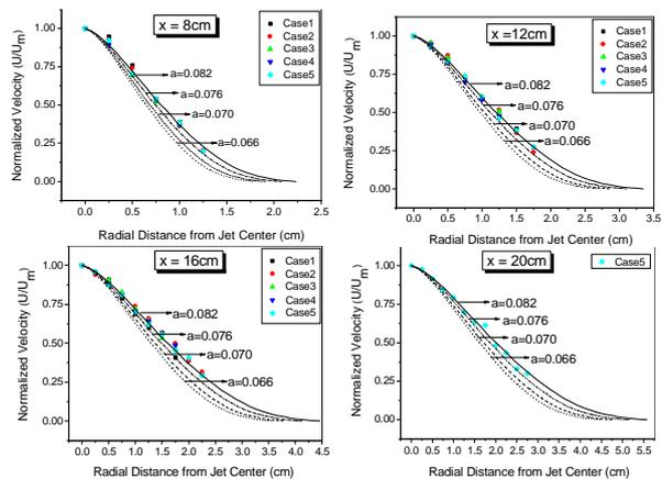
Figure 2. Velocity distribution of turbulent jet
