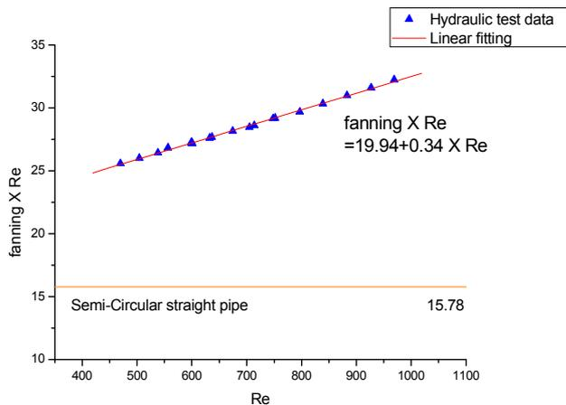
Figure 3. Fanning  $\times$  Re in terms of Re in the PCHE and semi-circular pipe
