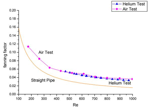
Figure 4. Fanning factors in terms of Re in helium test and air test using the KAIST PCHE
