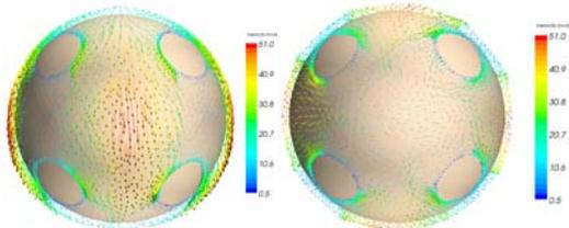
Fig. 3. Velocity vector around central pebble: (left) side view and (right) bottom view.
