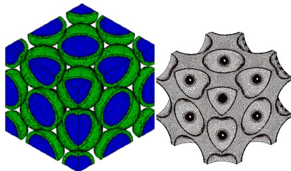
Fig. 2. Computational meshes for solid and fluid regions.
