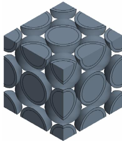
Fig. 1. Staggered pebble array model for CFD analysis.
