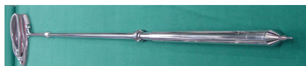
Figure 2. The 07M-21K irradiation capsule
