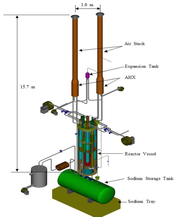
Fig. 2. Overall 3-dimensional schematic of test facility
