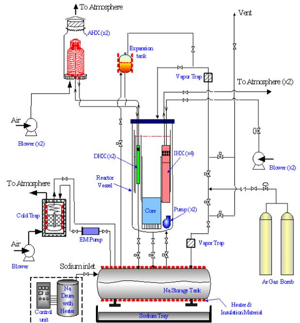
Fig. 1. Schematic diagram of test facility
