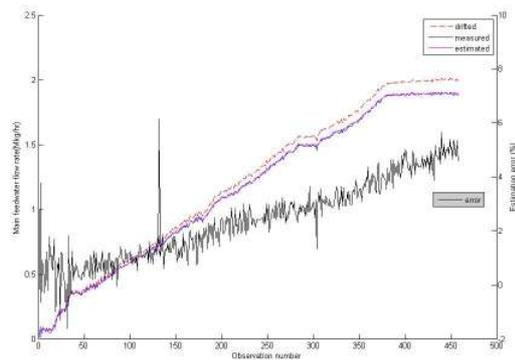
Fig. 4. Drifted signal and residual of estimate
