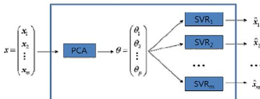
Fig. 1. The schematic diagram of PC-AASVR
