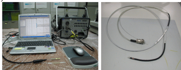
Fig. 1 MS-5800 ECT equipment and beaded bobbin type probe
