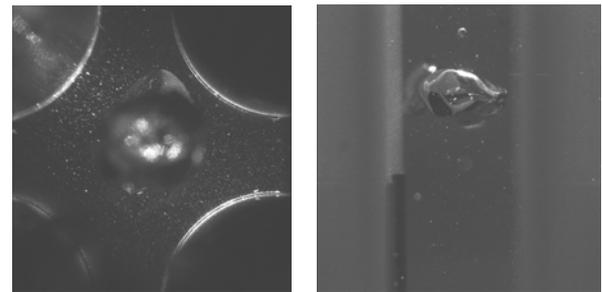
(b) Core peaking (bubble diameter ~ 8 mm)
