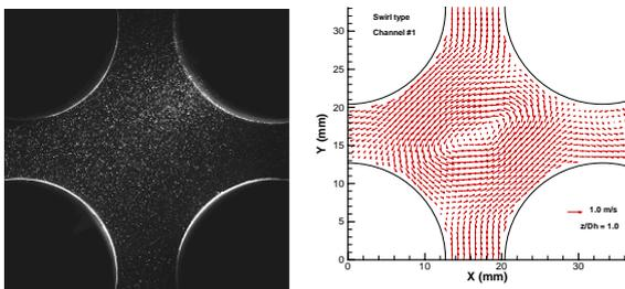
Fig. 3 Captured particle image (a) and the velocity vectors in a subchannel (b)
