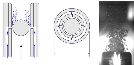
Fig. 2 Nozzle-type air/water injector
