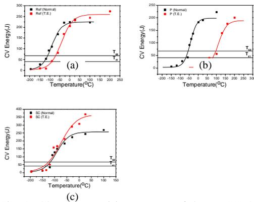
Fig. 2 Charpy transition curves of the (a) KL4-Ref, (b) KL4-P and (c) SC-KL4
