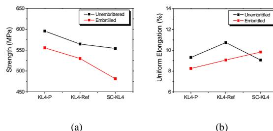
Fig. 1 Tensile test results of the model alloys.
