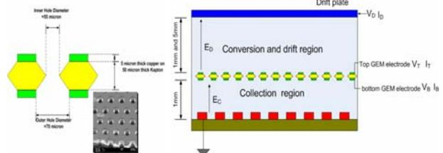
Fig. 2 schematic diagram of the single-GEM detector in this study
