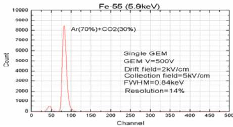
Fig. 3 Measured spectrum of X-ray from  $^{55}\text{Fe}$
