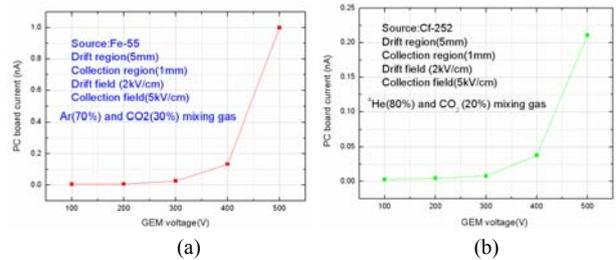
Fig. 4 GEM total gain as a function of  $\Delta V_{\text{GEM}}$  for X-ray (a) and fast neutron detection (b)
