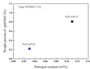
Fig. 3. Quantitative analysis of the precipitates in type 347 with respect to the Nitrogen content.
