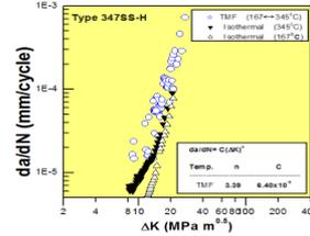
Fig. 5. Comparison of the obtained Thermo-Mechanical Fatigue crack growth rate with the Isothermal FCGR for type 347.
