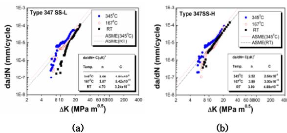
Fig. 4. The effect of temperature on FCGR in type 347. ; (a) SS-L , (b) SS-H
