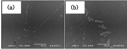
Fig. 2 SEM micrographs showing the precipitates in the 347 SSs ; (a) SS-L, (b) SS-H
