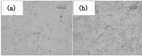
Fig. 1 Optical micrographs of type 347 SSs. ; (a) SS-L, (b) SS-H
