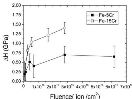
Figure 1 A change in the nano hardness of the irradiated Fe-5Cr alloy and the Fe-15Cr alloy with an irradiation fluence level.
