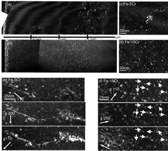
Fig.2 Cross-sectional view TEM micrographs of the irradiated Fe-5Cr alloy (a) and Fe-15Cr alloy (b), the evolution of irradiation induced dislocation loops in the Fe-5Cr alloy(c) and the Fe-15Cr alloy (d) at a depth of 1 $\mu$ m and weak beam dark-field micrographs of the irradiation induced dislocation loops with the reflections of  $g=110$ ,  $g=200$  and  $g=\bar{1}10$  in the Fe-5Cr alloy (e) and the Fe-15Cr alloy(f)
