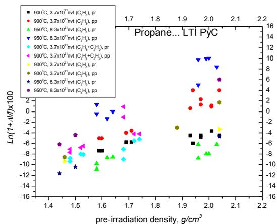
Fig. 4. Variation in lengths of PyC layer from propane as a function of pre-irradiation density (pr and pp mean parallel and perpendicular to the deposition direction, respectively).
