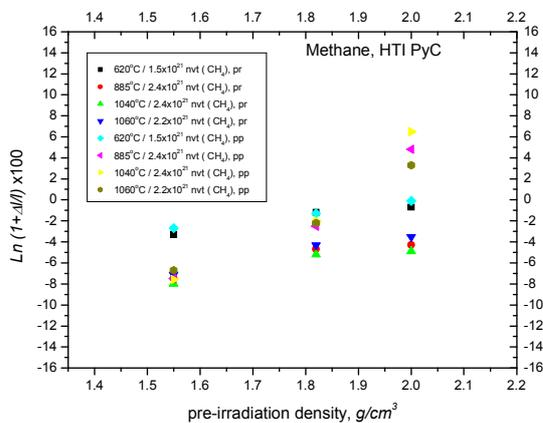
Fig. 3. Variation in lengths of PyC layer from methane as a function of pre-irradiation density (pr and pp mean parallel and perpendicular to the deposition direction, respectively).
