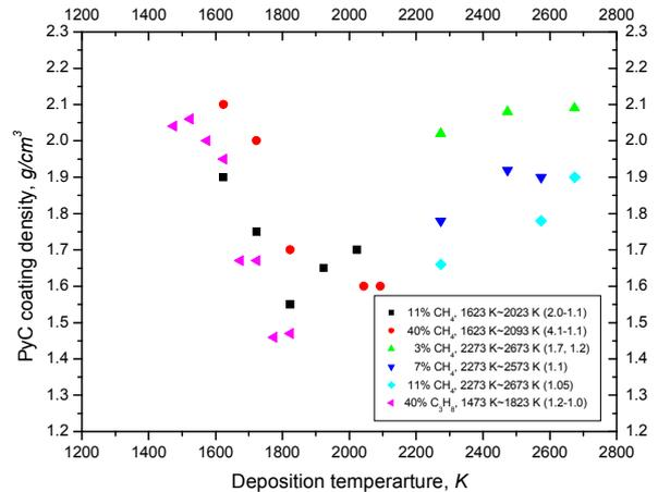
Fig. 1. Variation of PyC coating density as a function of deposition temperature.
