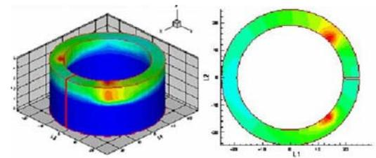
Fig. 6 Steam fraction in IRWST after accident (100s later)
