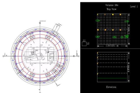
Fig. 2 Division concept(L) and 3-D model(R) for IRWST of APR1400
