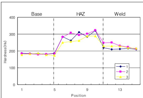
Figure 5. Hardness(applied load : 10kg)
