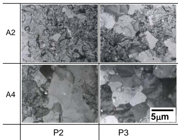
Fig. 2. TEM micrographs of the HANA-6 alloy with different manufacturing parameters after the final steps
